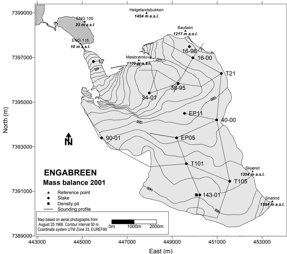
Figure 3. Sounding profiles and stakes used for velocity measurements in Engabreen, Svartisen, Norway in 2001.
