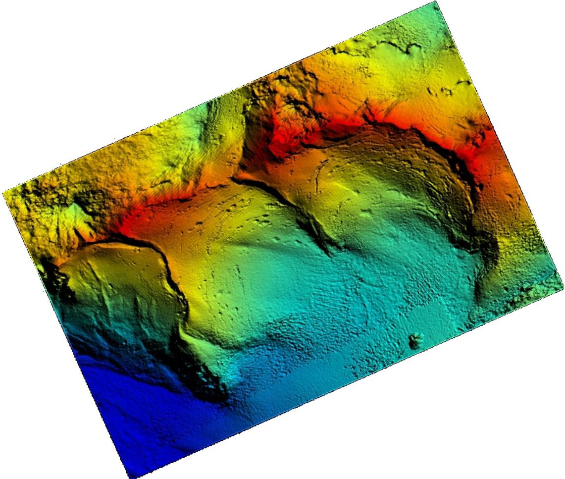
*Figure 9. Digital elevation model generated over Svartisheibreen, Svartisen, Norway using digital camera imagery applying global block adjustment approach, 24 September 2001 .*
